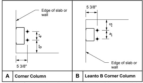
Installation of concrete anchors will require special inspection. Holes must be drilled with a specific drill bit, as noted on the engineering plans.
