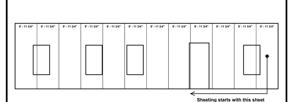
This illustration is for reference only, and is to be used to supplement the engineering drawings. If any discrepancies occur, the engineering plans will always take precedence.
