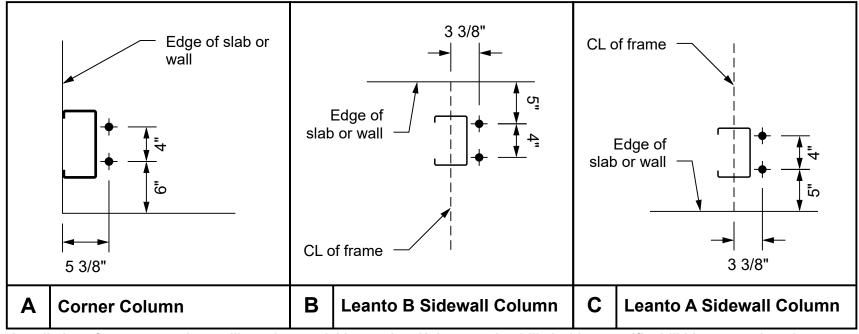
Installation of concrete anchors will require special inspection. Holes must be drilled with a specific drill bit, as noted on the engineering plans.
