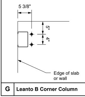
Installation of concrete anchors will require special inspection. Holes must be drilled with a specific drill bit, as noted on the engineering plans.
